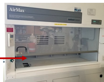
White bucket is barely visible through the sash due to etching.
