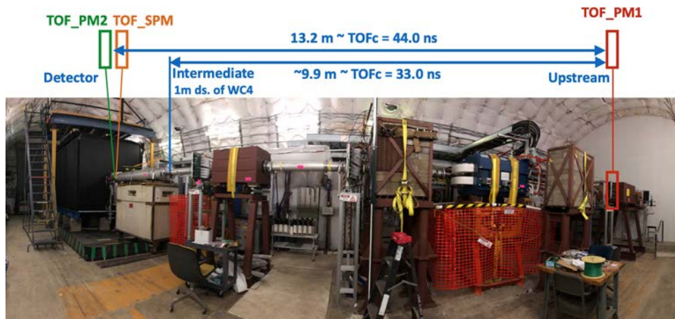
Figure 4.1: The pre-redeployment configuration of the ToF detectors. TOFc is the time it would take light to travel the indicated pathlength, to be interpreted as an estimate of the time of flight of fast particles. Slide: Alex Sousa, docdb-48480
