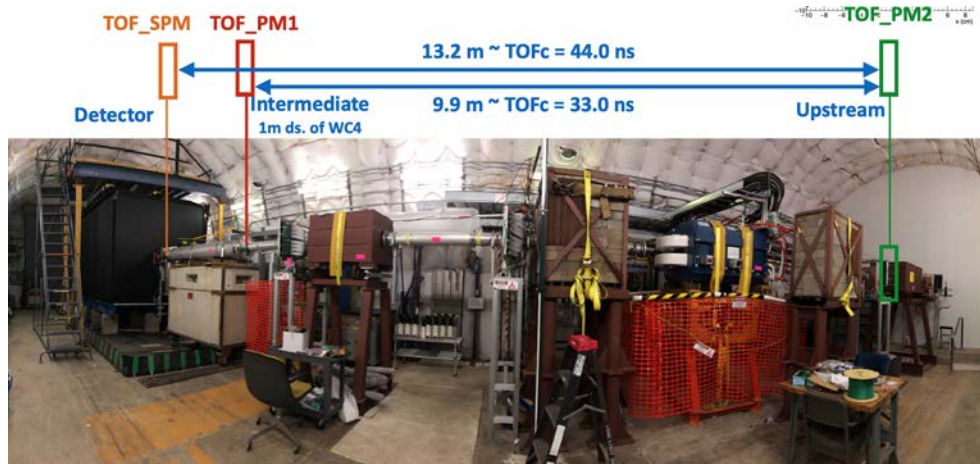
Figure 4.2: The post-redeployment configuration of the ToF detectors. TOFc is the time it would take light to travel the indicated pathlength, to be interpreted as an estimate of the time of flight of fast particles. Slide: Alex Sousa, docdb-48480
