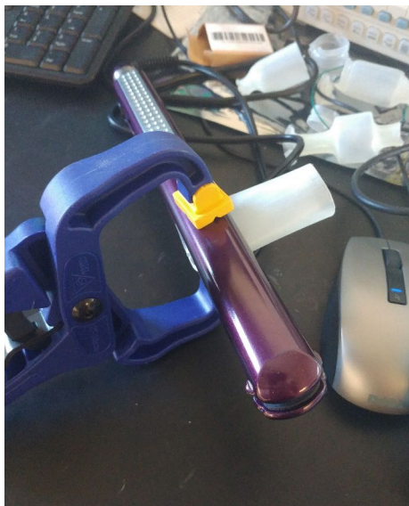
Figure 4.2: Flat Iron Heat Shrink Tube Setup
