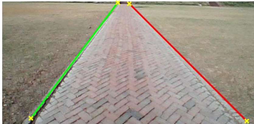
Figure 3.8: The line data retrieved from the Hough transform is plotted over the cropped image from Figure 3.1(b) demonstrating the edges of the path were successfully found.
