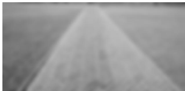
Figure 3.4: The image from Figure 3.3 is blurred using a 2D Gaussian filter. Notice the distinction between the dark sections of ground and lighter section of the path.
