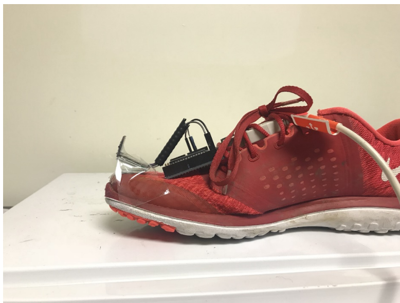
Figure 5.16: Sensor on shoe, angle was set by fastening the sensor to a piece of metal.
