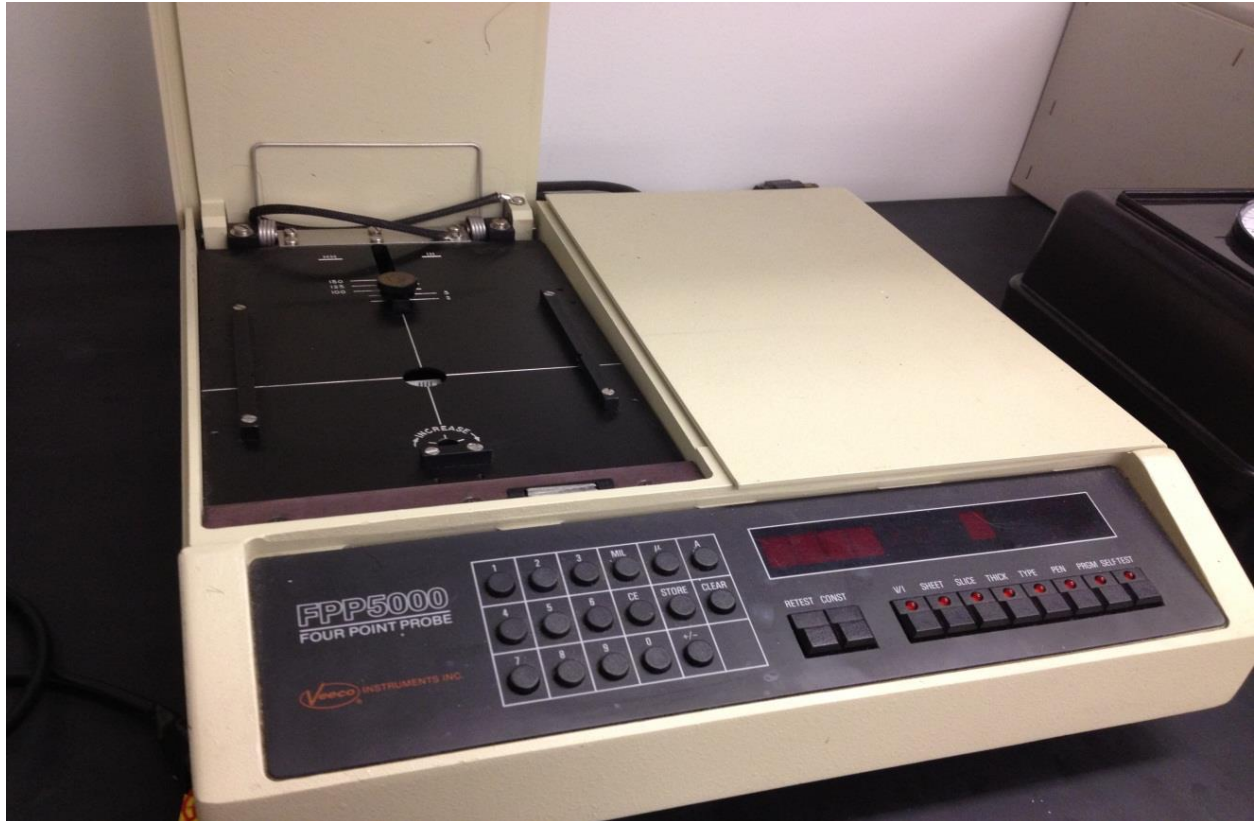
Figure 2: Four-Point Probe; current is measured across two points and voltage is measured across the other two, forming a simple circuit. Each contacts the surface of the thin film and the device uses Ohm's law to calculate sample resistance.
